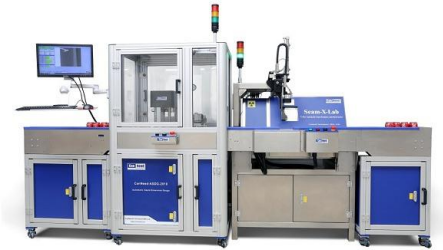
Seam-X®-Line X-Ray Automatic Seam Scanner (Non-destructive+Auto sampling)
